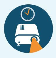
Use a new lamp more intensively than usual, any malfunction generally occurs during the first 10 hours of operation. We recommend that schools and businesses which stock replacement lamps test each lamp by using it for at least 20 hours.
