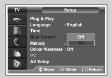
If no signal is being received or the signal is very weak, a blue screen automatically replaces the noisy picture background. If you wish to continue viewing the poor picture, you must set the "Blue Screen" mode to "Off".
