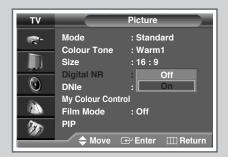
If the signal received by your television is weak, you can activate this feature to help reduce any static and ghosting that may appear on the screen.
