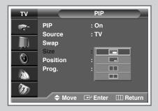
You can display a sub picture within the main picture of TV program or external A/V devices. In this way you can watch TV program or monitor the video input from any connected devices while watching TV or other video input.
