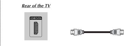
The "HDMI/DVI IN" does not support the Analog R (red), G (green) and B (blue) signals.
