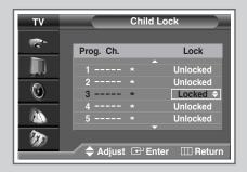
This feature allows you to prevent unauthorized users, such as children, from watching unsuitable programmes by muting out video and audio. Child Lock cannot be released using front panel buttons. Only remote control can release the Child Lock setting, so keep the remote control away from children.
