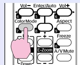
Each time you press the button, the color mode name is displayed on the screen and the color mode changes.
