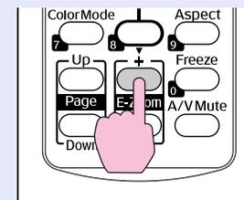
Each time the button is pressed, the area is expanded. You can expand quickly by holding the button down. You can reduce the enlarged image by pressing the [-] button. Press the [Esc] button to cancel.
